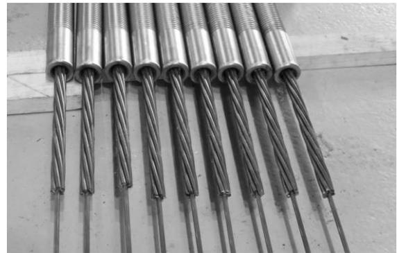
Fig. 1 Anchorage condition of the testing cable
