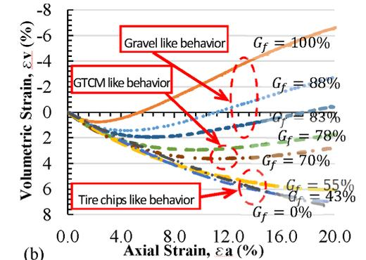
Fig3. (a) Deviatoric stress-axial strain (b) Volumetric strain -axial strain relation of GTCM at different gravel fraction ( $D_r = 50\%$ ,  $\sigma_3 = 100$  kPa)
