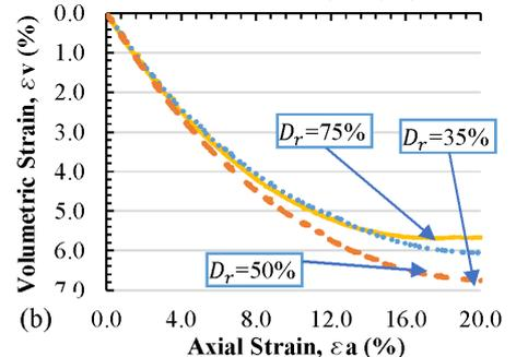
Fig5. (a) Deviatoric stress-axial strain (b) Volumetric strain -axial strain relation of GTCM at different relative density ( $G_f = 55\%$ ,  $\sigma_3 = 100$  kPa)
