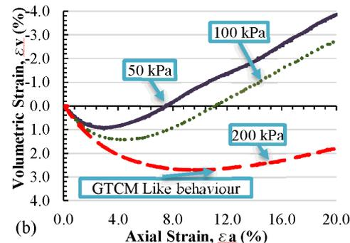
Fig4. (a) Deviatoric stress-axial strain (b) Volumetric strain -axial strain relation of GTCM at different confining pressure ( $D_r = 50\%$ ,  $G_f = 88\%$ )
