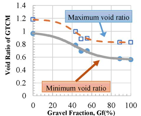
Fig2. Maximum and minimum void ratio of GTCM
