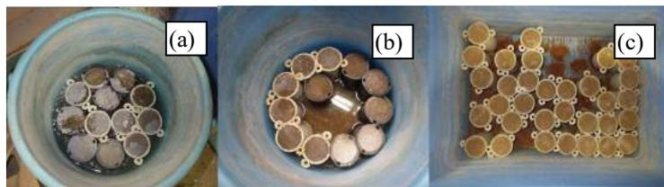
Fig.2: Test Sample condition: (a) Cement, (b) Quick Hardening cement, (c) Lime treated samples.
