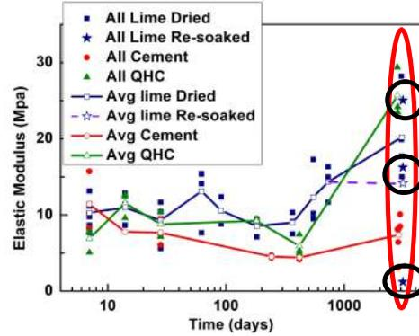
Fig. 4 Elastic Modulus vs Elapsed Time. (Ref to Fig. 3)
