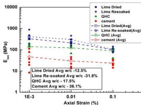
Fig. 6  $E_{sec}$  vs Axial Strain
