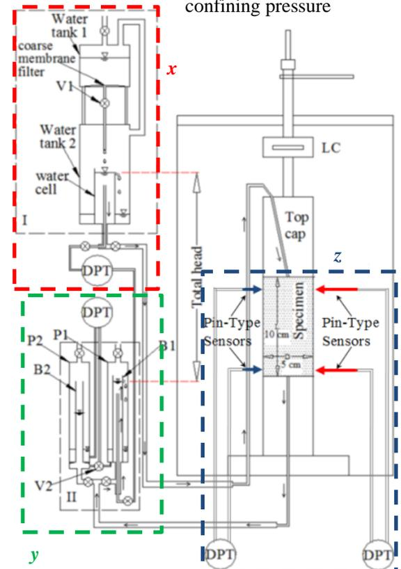
Fig.2 Schematic Diagram of Triaxial Apparatus w/ two sets of pin-type sensors
