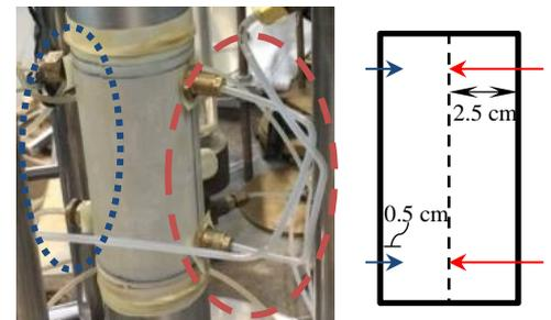
Fig.3 Two sets of pins, one set at 2.5 cm length while another is 0.5 cm
