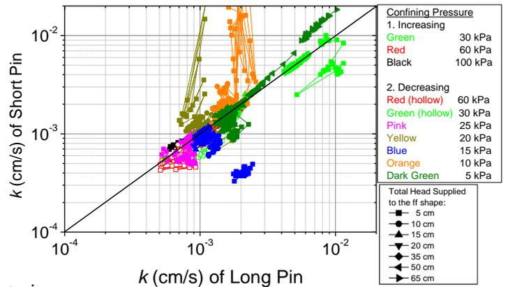
Fig.4 Comparison of  $k$  of long and short pins
