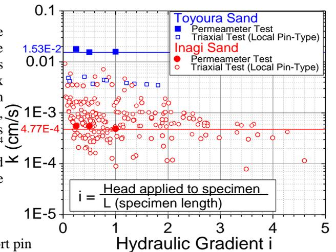
Fig.6 Comparison of  $k$  between Permeameter Test and Triaxial Test (Local Pin-Type)
