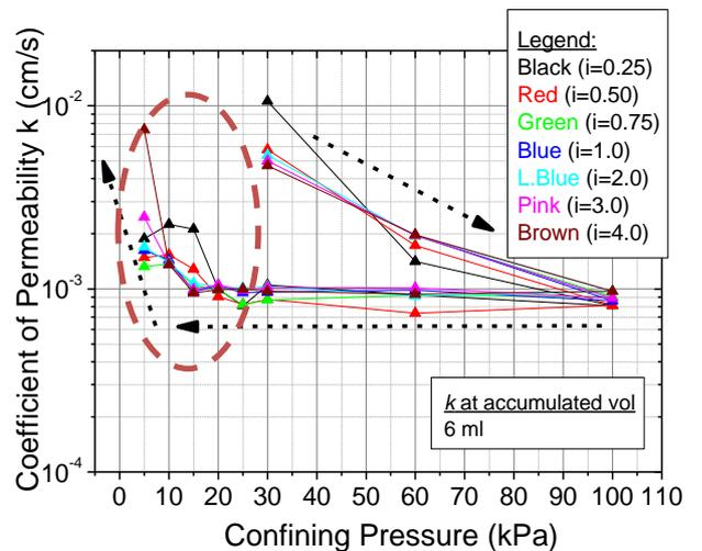
Fig.5 Effect of Confining Pressure on  $k$
