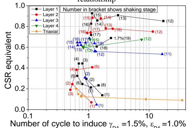
Fig. 6 CSR-Number of cycle to liquefy relationship
