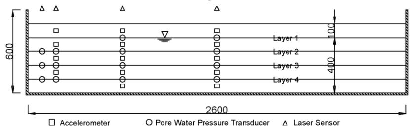
Fig. 2 Shaking table model and instrument arrangement (unit in mm)
