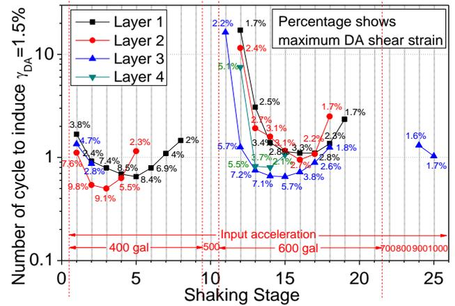
Fig. 5 Liquefaction resistance-shaking stage relationship
