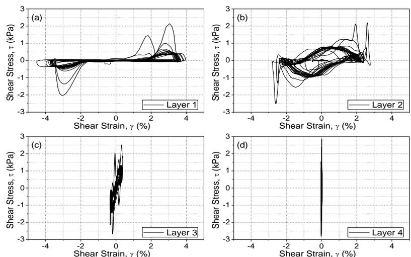
Fig. 4 Shear stress-strain relationship of layer 1(a), 2(b), 3(c) and 4(d)
