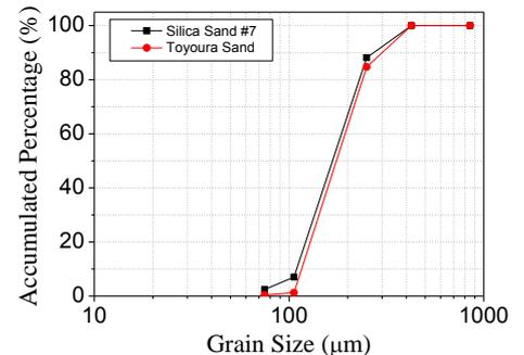
Fig. 1 Gradation of Silica Sand No.7
