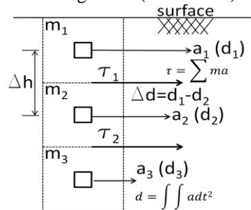
Fig. 3 Computation of shear stress and shear strain
