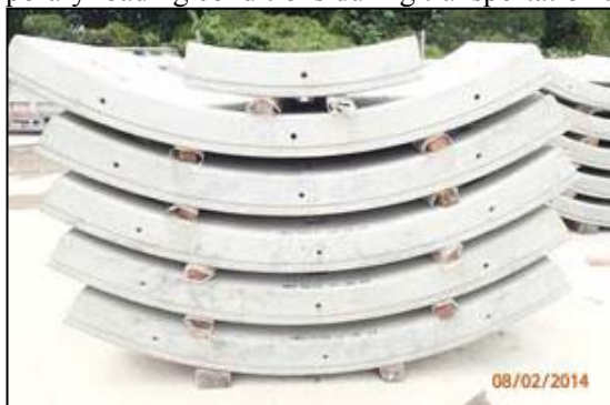
Figure 4 RC Segment Lining
