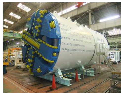
Figure 2 EPB TBM for Tunnel Excavation
