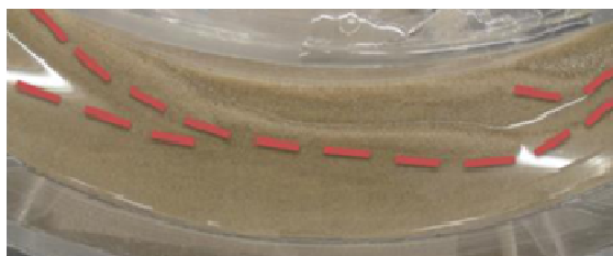
Fig. 2 Channel between adjacent point bars. The main flow is from left to right.
