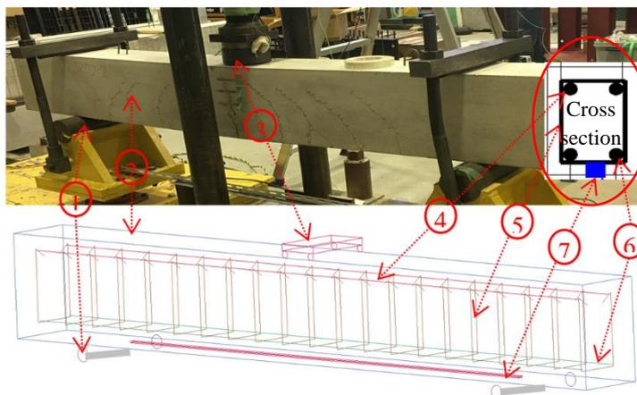
1: Supports, 2: Concrete, 3: Load cell, 4: Top bending bar, 5: Shear reinforced bar, 6: Bottom bending bar, 7: Carbon fiber
