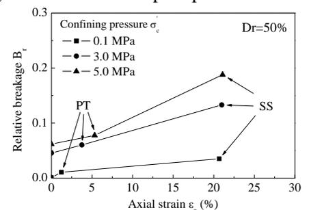
Fig.3 Br plotted against the axial strain
