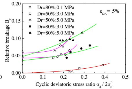
Fig. 6 Br plotted against cyclic deviatoric stress ratio
