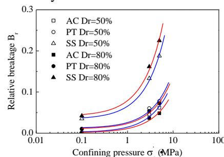
Fig.2 Br after several stages of Aio sand in monotonic tests
