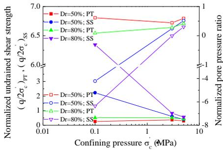
Fig. 4 Normalized undrained shear strength and pore pressure ratio plotted against confining pressure
