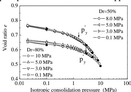
Fig.1 Isotropic compression curves of Aio sand
