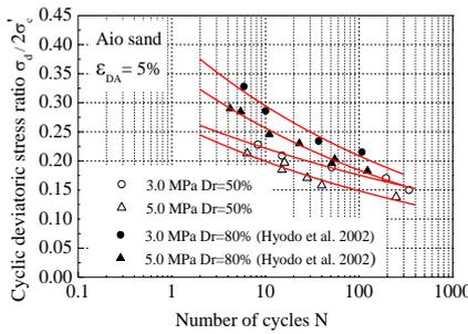
Fig. 5 Liquefaction resistance strength
