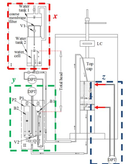
Fig.3 Schematic Diagram of Triaxial Apparatus with Confining Stress at the specimen
