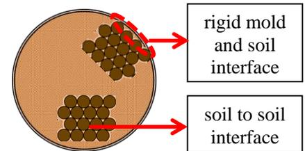
Fig.1 Schematic Cross Section of Rigid Mold using JIS A 1218
