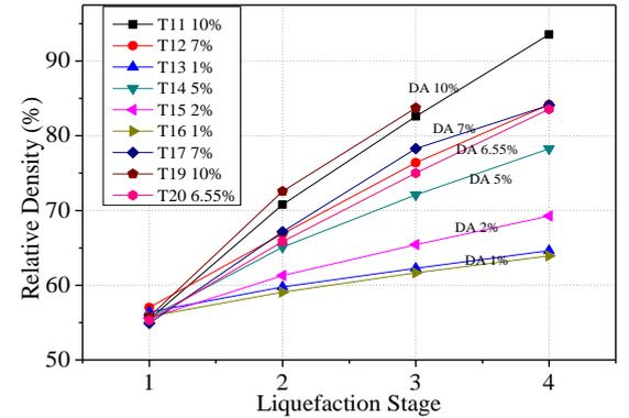
Fig.4 Relative Density Change during Repeated Liquefaction Test
