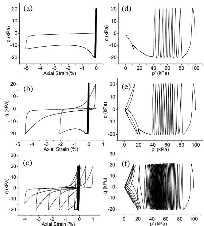
Fig.2 Stress-Strain Relationship of Stage 1 (a), 2 (b) and 3 (c) and Effective Stress Path of Stage 1 (d), 2 (e) and 3 (f)
