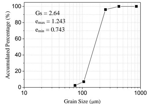
Fig.1 Gradation of Silica Sand No.7
