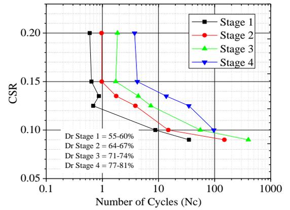
Fig.3 Repeated Liquefaction Curve
