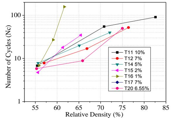
Fig.6 Liquefaction Resistance versus Relative Density of 3 Stages
