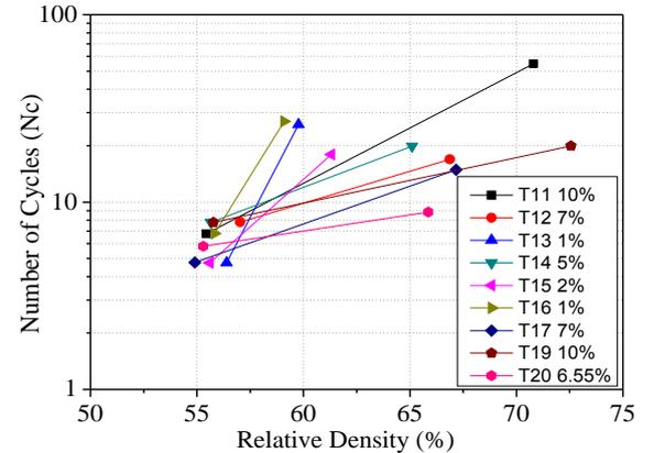
Fig.5 Liquefaction Resistance versus Relative Density of 2 Stages
