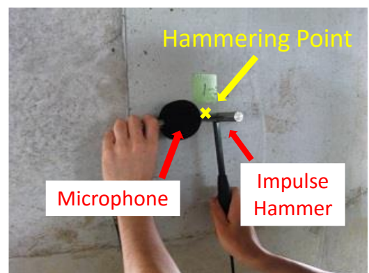
Photo 3 Impulse Hammering Test
