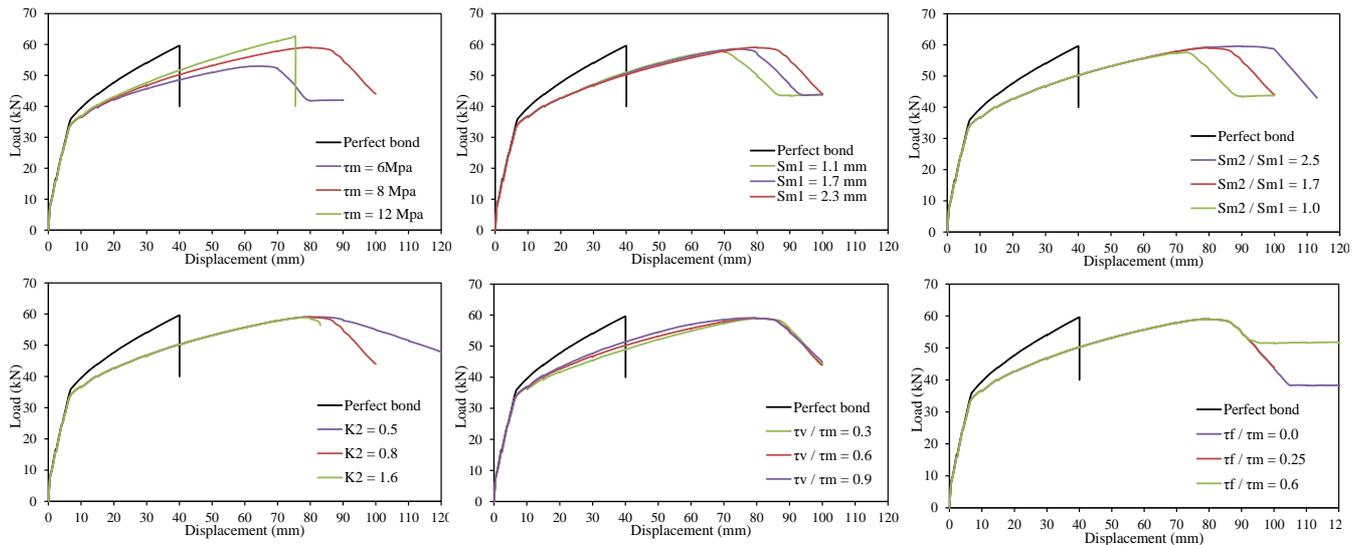
Fig. 2 Effect of bonding parameters of BFRP bars on the load-displacement relation of FSRC column
