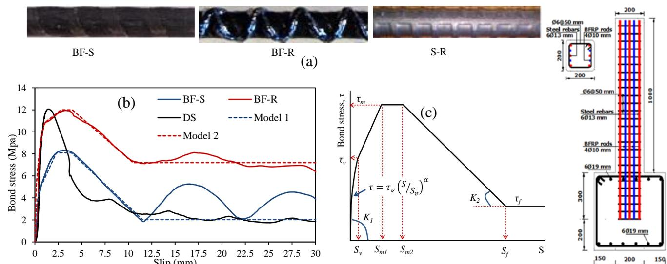
Fig. 1 (a) Surface texture configurations of BFRP and steel bars, (b) Bond-slip relationships resulted from pull-out tests, (c) Proposed bond-slip model for BFRP bars, and (d) Dimensions and reinforcement details of the FSRC column
