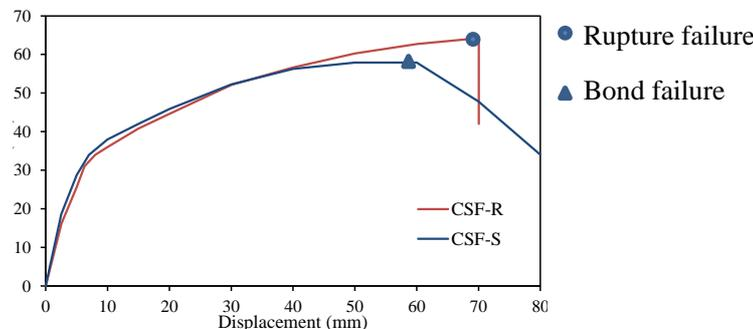
Fig. 3 Experimental load-displacement relations of columns reinforced by BFRP bars with surface texture BF-S (column CSF-S) and surface texture BF-R (column CSF-R)
