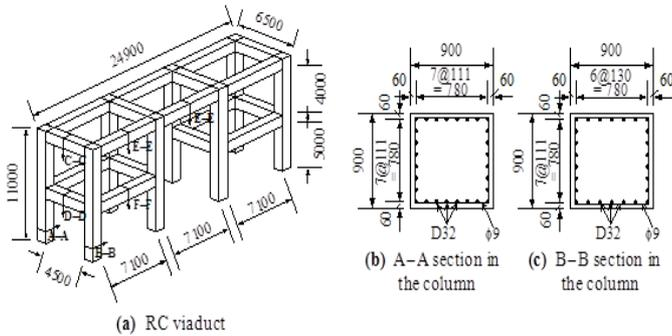
Fig. 3 Target structure details
