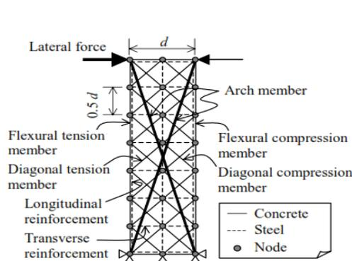
Fig. 1 2D lattice model for columns (Miki et al. 2004)
