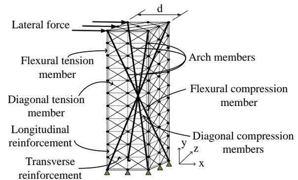
Fig. 2 3D lattice model for columns (Miki et al. 2004)
