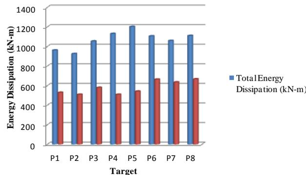
Fig. 5 Energy dissipation in Hansui R5 viaduct columns
