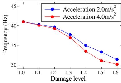
Fig. 2 Damage level versus natural frequency in beam model
