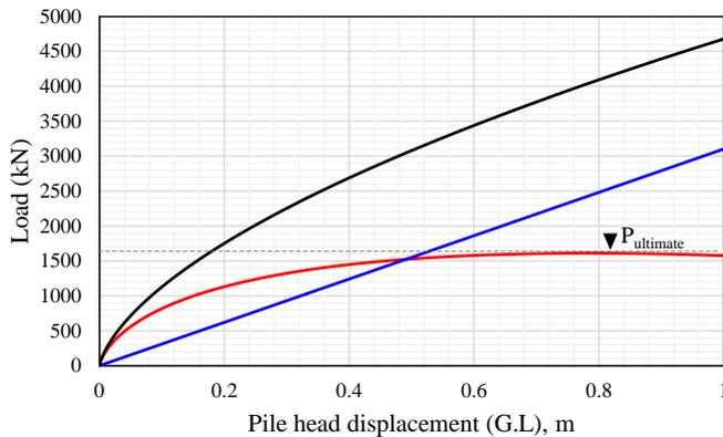
Fig. 2. Load-Deformation Curve for  $d=0.30\text{m}$   $E_p=200\text{GPa}$
