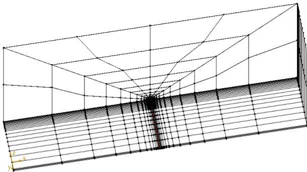
Fig. 1 3D Soil-Pile Configuration System
