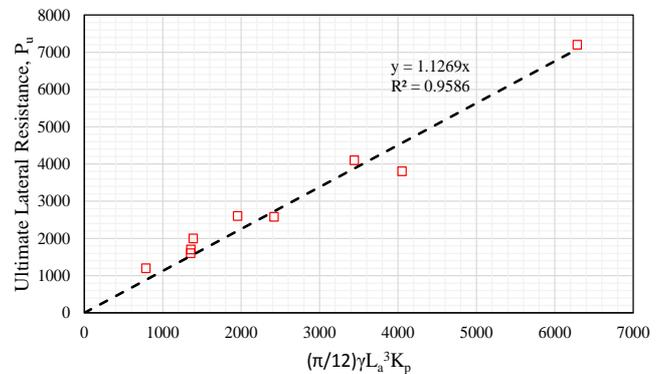
Fig. 4. Relationship of  $P_u$  with  $\gamma K_p L_a^3$
