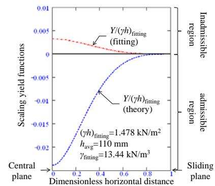
Fig. 2 Distribution of scaling yield functions along dimensional horizontal distance
