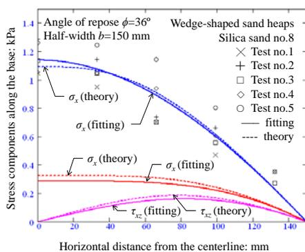
Fig. 1 Comparison between profiles of stress components and experimental vertical stress acting along a half-width base of sand heaps
