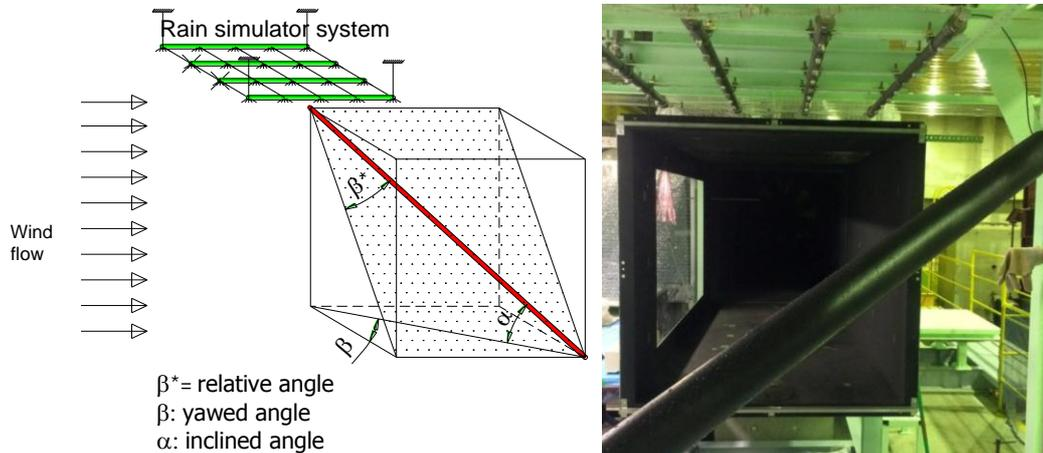
Fig. 3 The Wind tunnel test with rain simulator
