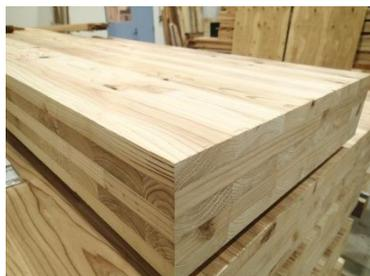
写真-1 CLT (直交集成板)
