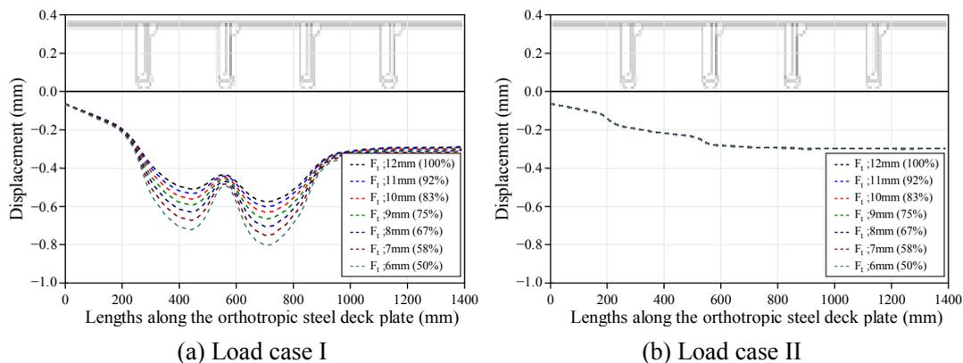
Figure 2 Displacement distributions on lower surface
