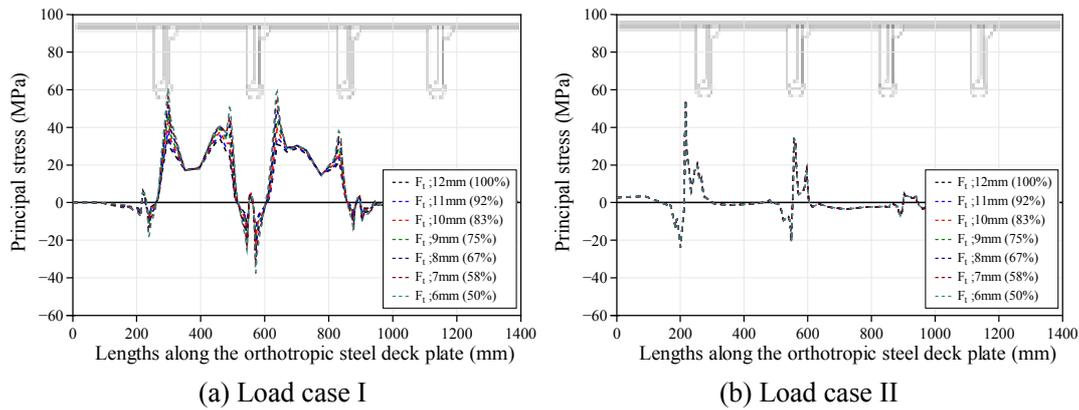
Figure 3 Stress distributions on lower surface
