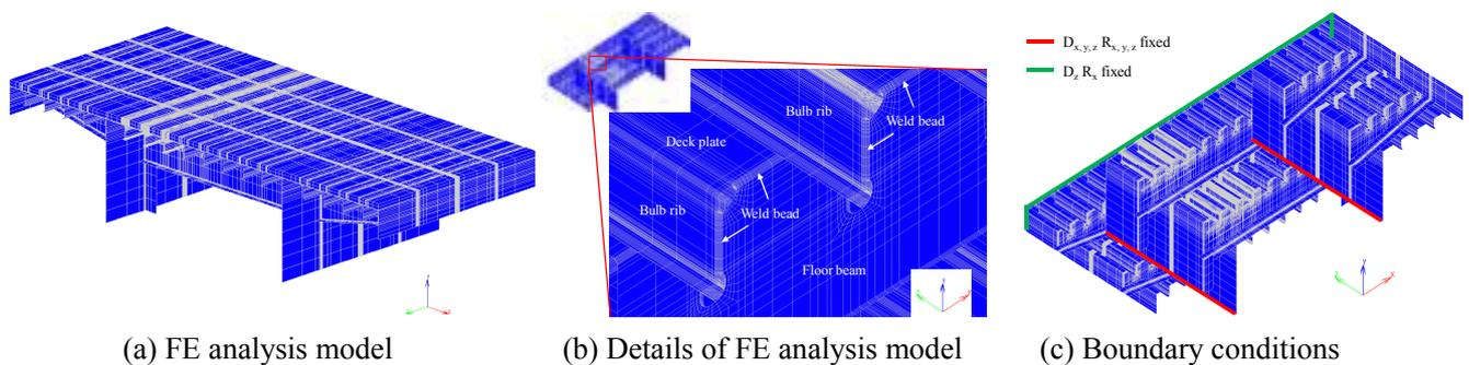
Figure 1 Details and boundary conditions of FE analysis model
