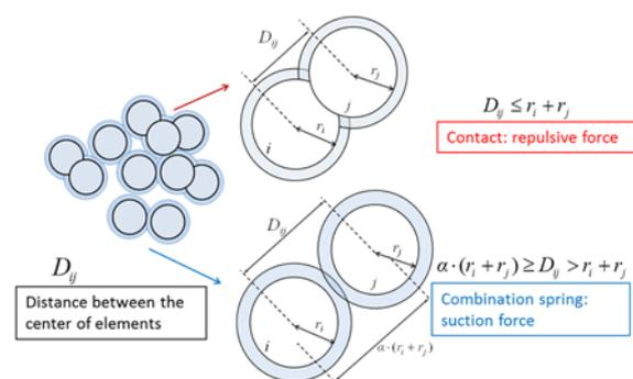
Fig.2 Modeling of suction effect by virtual water screen
