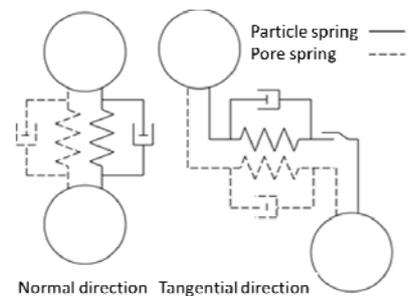
Fig.1 Modeling of interaction between elements by EDEM
