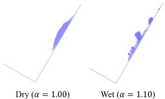
Fig.5 Simulation results of flow state (0.4 (s))
