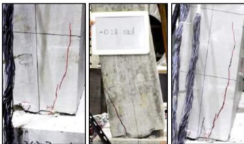
Photo 1 Failure mode for basic specimen with plain bar
