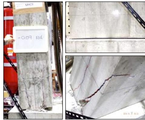
Photo 2 Failure mode for basic specimen with deformed bar
