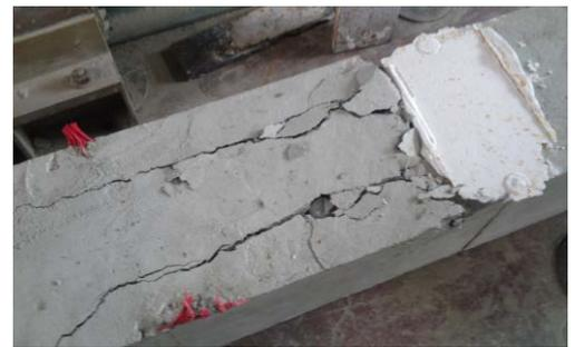
写真-1 供試体上面のひび割れ (No. 1)
