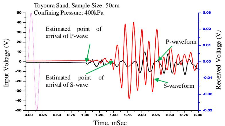
Fig. 5: typical received waveform
