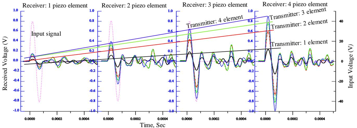
Fig. 4: Received S-wave signal at receiver and transmitter disk are facing each other, input sine 10 kHz
