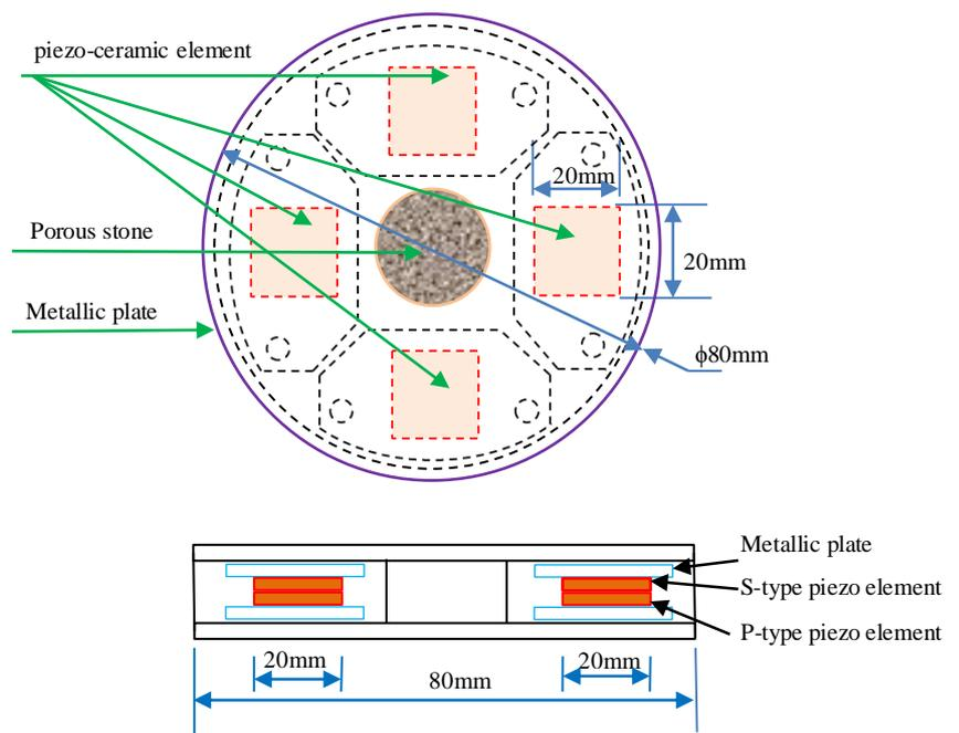
Figure 3: Schematic diagram of large size flat shaped disk transducer
