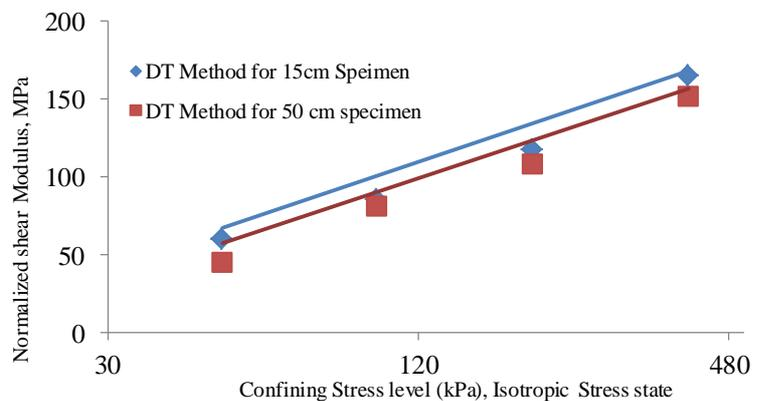
Fig. 6: comparison of Normalized shear modulus of toyoura sand in different specimen length
