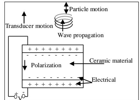
Figure 2: sketch of P-type element
