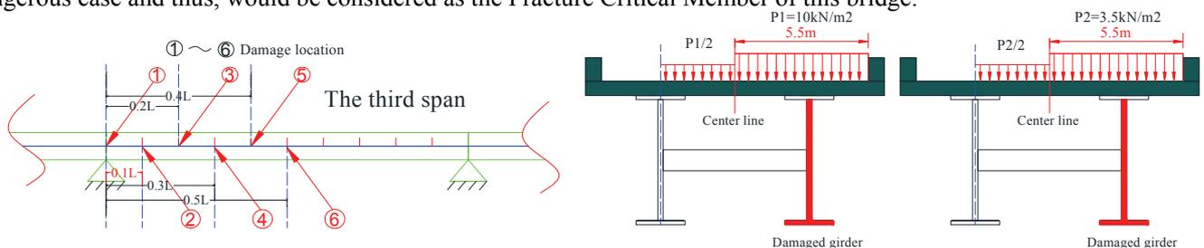
Figure 2: Loading conditions and damaged positions
