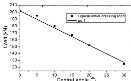
(a) Initial cracking load
