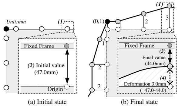
Fig.5 Method for deformations of sections
