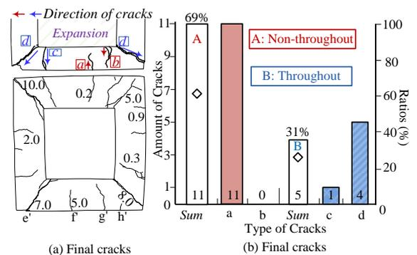
Fig.3 Cracks in upper side
