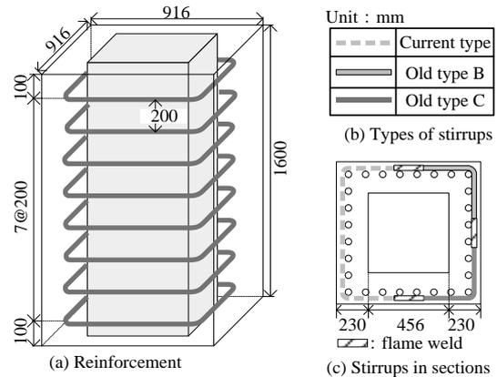
Fig. 1 Shape of Specimen
