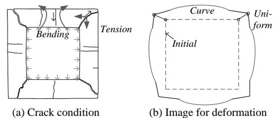
Fig.4 Cracks related to deformations
