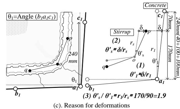
Fig.6 Deformations for stirrups and concrete
