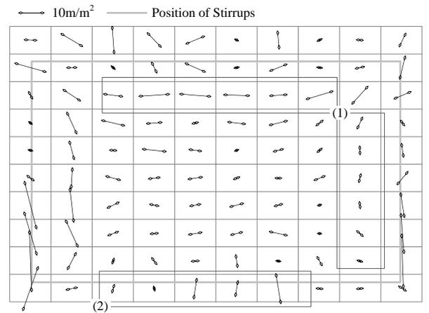
Fig. 6 Crack Density and Directions
