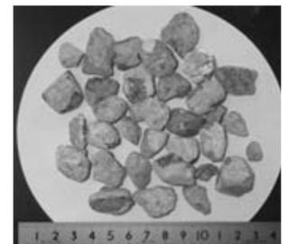
写真-2 再生粗骨材 M (DM)
