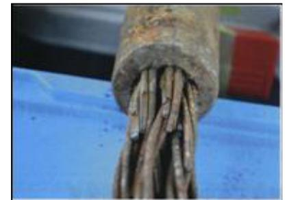
写真-5 PC 鋼線破断事例<sup>4)</sup>
