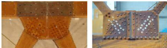
(a) P25d (b) P72u Photo 1: Gusset plate connections
