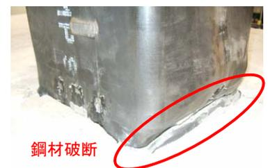
図4 鋼材破断状況(No. 2-1)
