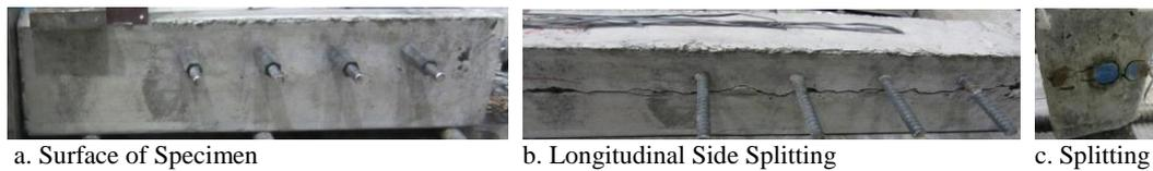
**Fig.8 Surface before and after testing with fracture pattern (Case-2)**
