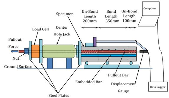
**Fig.5 Loading Arrangement**
