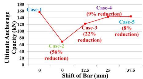
**Fig.7 Ultimate anchorage capacity - shift of bar**
