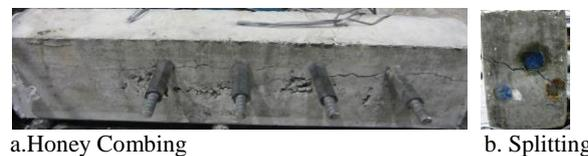
**Fig.9 Fracture Pattern (Case-5)**
