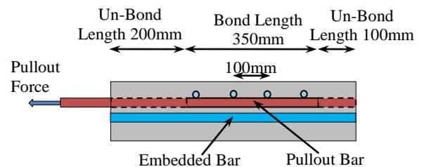
Fig.4 Side View of Specimen
