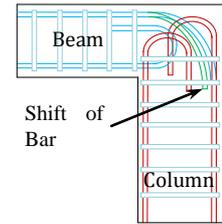
Fig.1 Typical Beam Column Joint
