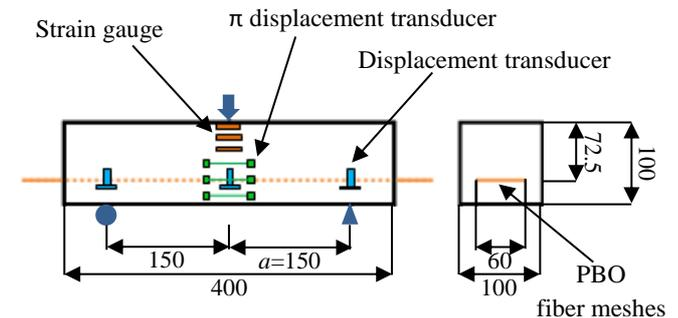
Fig. 3 Detail of specimens (unit: mm)
