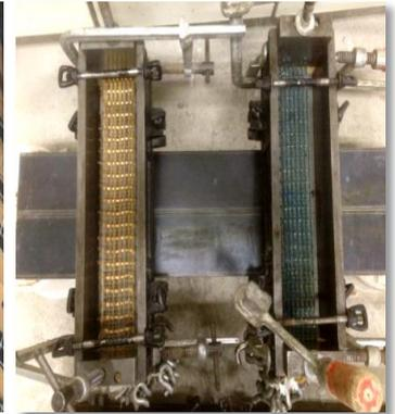
Fig. 1 PBO fiber meshes Fig. 2 Formwork preparation
