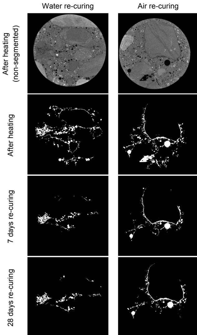
Figure 2 Cracks after heating and re-curing
