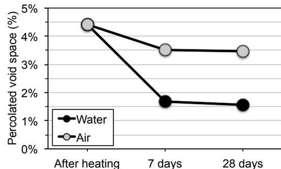
Figure 4 Change in crack volume due to re-curing
