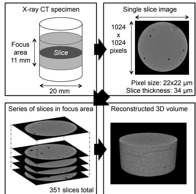
Figure 1 Image acquisition and 3D reconstruction details
