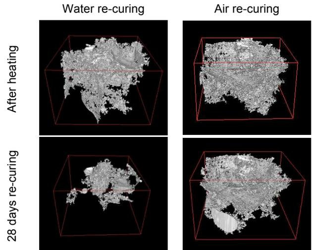
Figure 3 Three-dimensional crack networks
