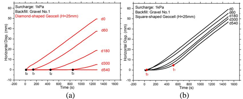
**Fig.4** Horizontal displacement along the geocell reinforcements versus time history: (a) diamond-shaped geocell; (b) square-shaped geocell
