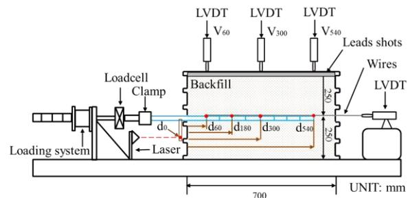
Fig.1 Schematic diagram of pullout test apparatus
