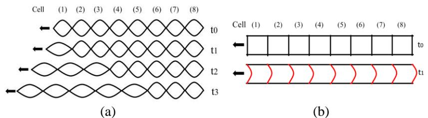
**Fig.5** Schematic diagram of deformation status vary with time: (a) diamond-shaped geocell and (b) square-shaped geocell
