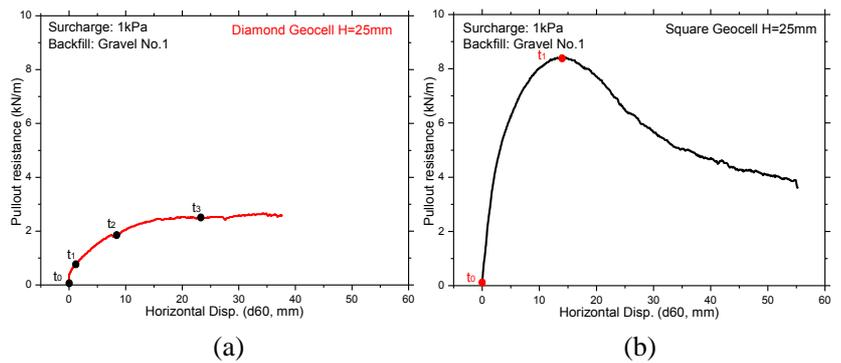
**Fig.3** Pullout resistance against horizontal displacements ( $d_{60}$ ): (a) diamond-shaped geocell; (b) square-shaped geocell
