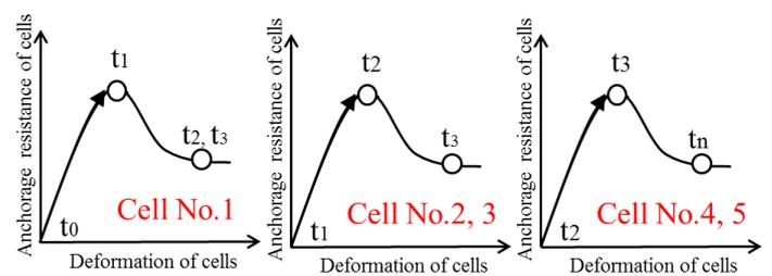
**Fig.6** Schematic diagram of stress-deformation mechanism of diamond-shaped geocell
