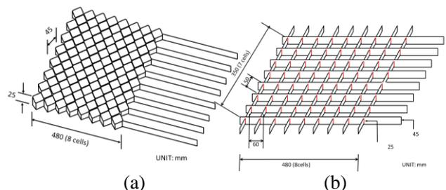
Fig.2 Geometry characteristics of: (a) diamond-shaped geocell and (b) square-shaped geocell
