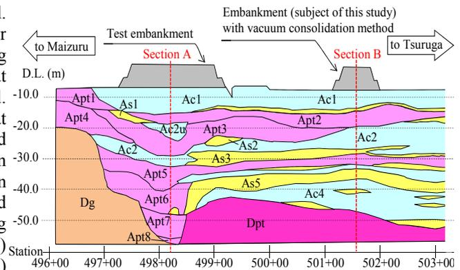
Fig. 1. The schematic outline of soil strata in Mukasa area (longitudinal section)
