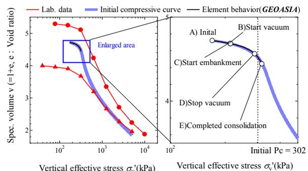
Fig. 6. Behavior of elements in layer Dpt1 under embankment center
