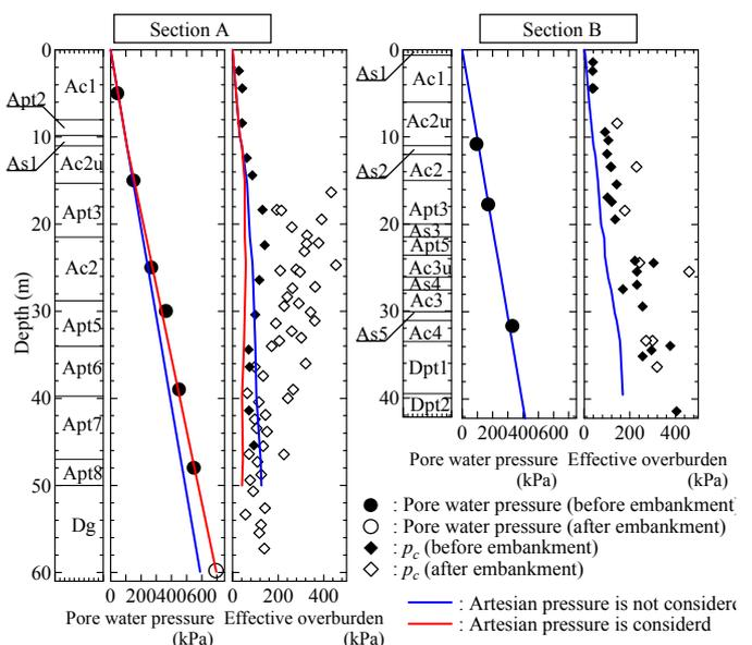
Fig. 3. Estimated distributions of initial pore water pressure and effective overburden pressure
