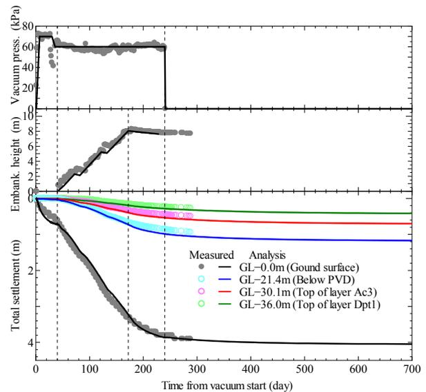
Fig. 5. Settlement under the embankment center
