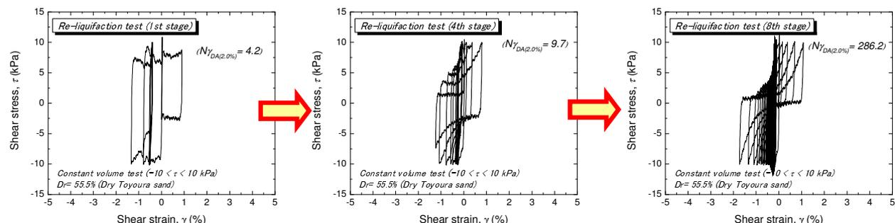
Fig. 2: Typical results of a re-liquefaction test at stages 1, 4 and 8 (Stages 2, 3, 5, 6, and 7 are skipped)
