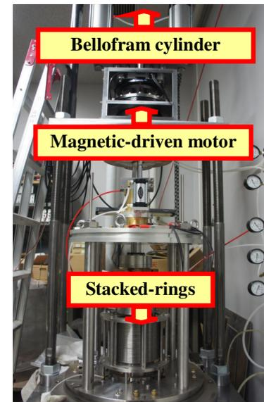
Fig. 1: Stacked-rings shear apparatus
