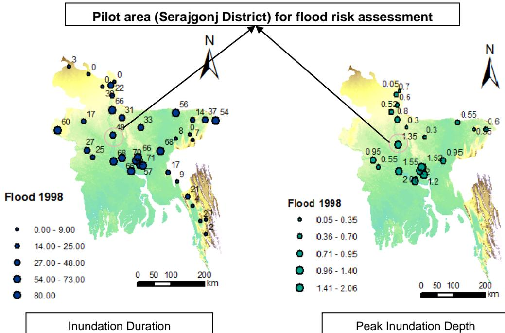
Figure 1: Peak inundation duration in days (left) and peak inundation depth in meters (right) during 1998 flood.
