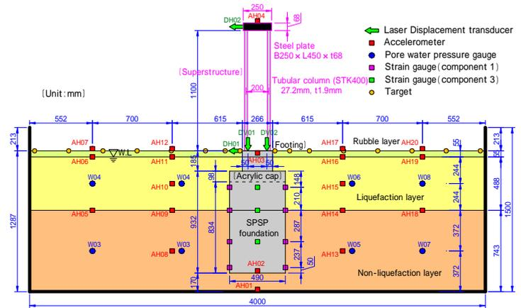
Fig-1 Physical model and instrument arrangements
