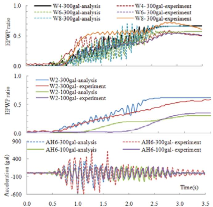
Fig-2 EPWP ratio and acceleration response of ground
