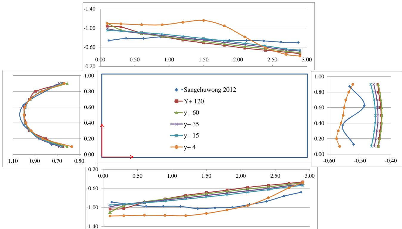
Figure 1. Pressure Coefficient ( $C_p$ ) plot around the cylinder for various  $y^+$  value.
