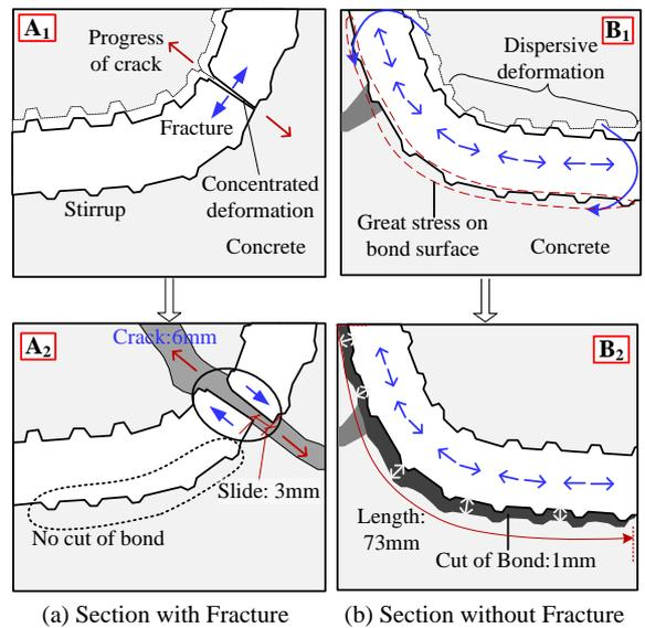
Fig. 6 Image of Mechanism
