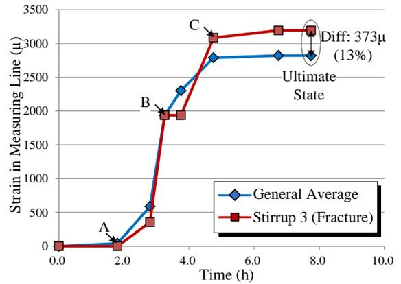
Fig. 4 Comparison of Strain in Measuring Line
