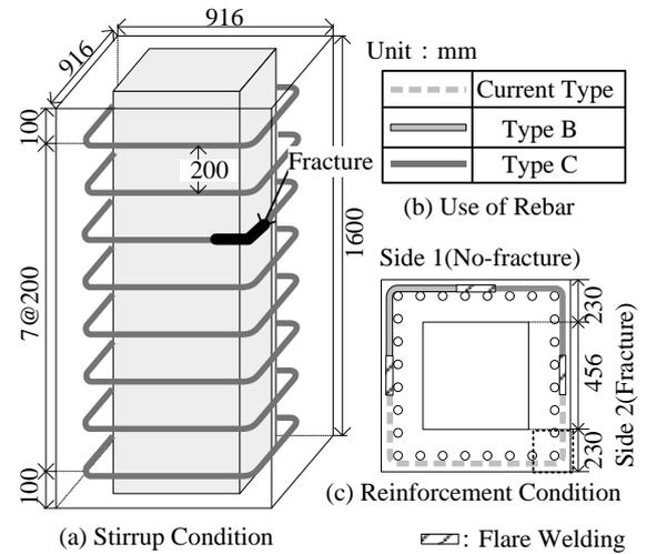
Fig. 1 Shape of Specimen & Fracture Position
