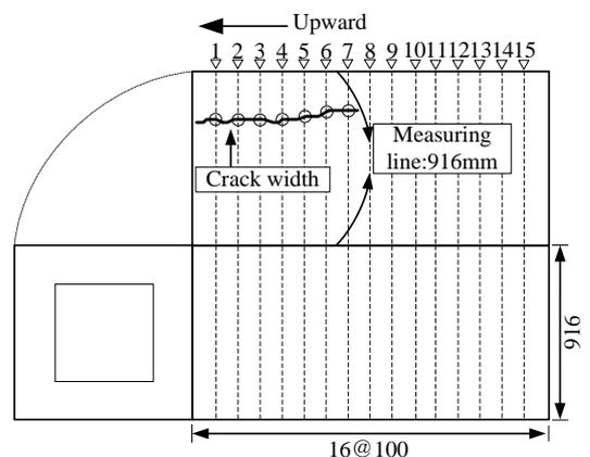
Fig. 3 Measurement of Strain
