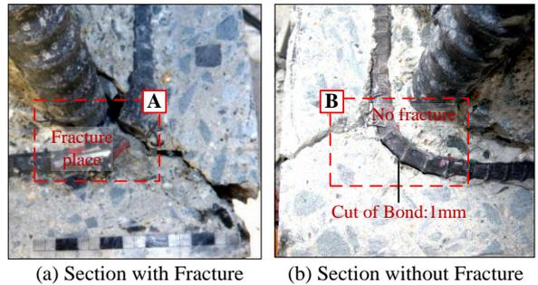
Fig. 5 Fracture Part & Non-fracture Part
