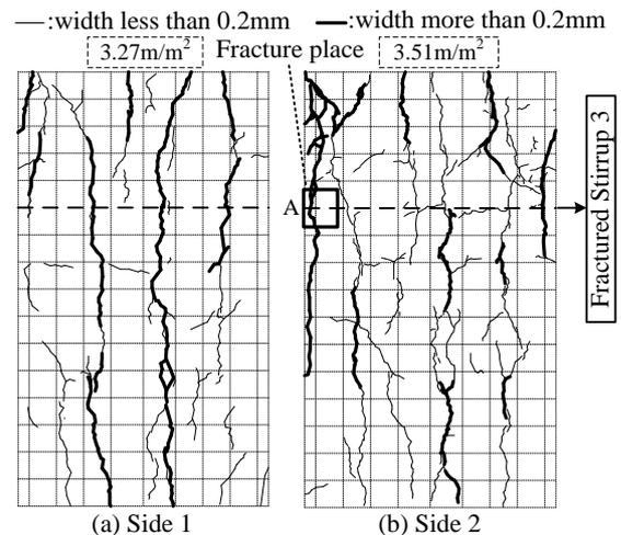
Fig. 2 Ultimate Crack Condition (Side 1, 2)
