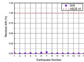
Fig. 5 Residual deformations under MCE-level ground motions
