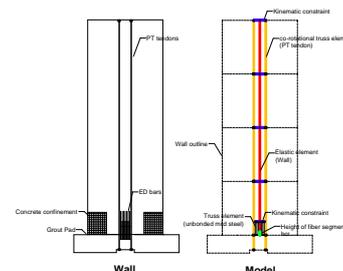
Fig. 2 Schematic of the wall and improved OpenSees model diagram of the wall
