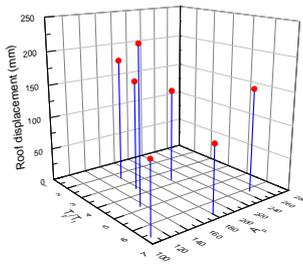
Fig. 6 Correlation of the peak story displacement demand with the pulse characteristics of near-fault ground motions.
