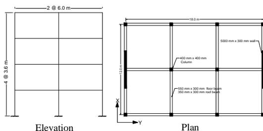
Fig. 1 Elevation and plan view of the prototype building
