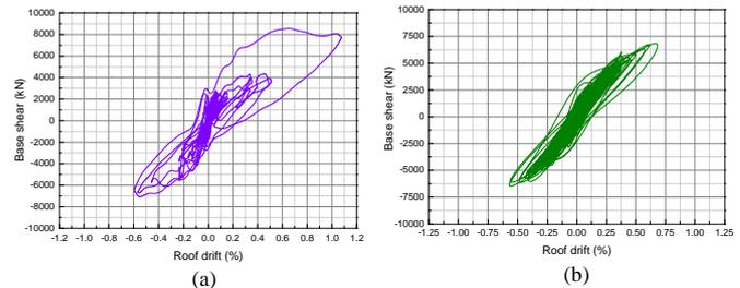
Fig. 7 Typical base shear vs. drift demand for MCE-level ground motions: (a) EQ. 181; (b) EQ. 169
