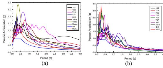
Fig. 3 Comparison of 5%-damped response spectra of ground motions with the target spectra: (a) near-fault (b) far-fault
