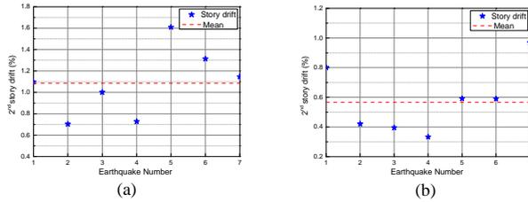
Fig. 4 Story drift results: (a) near-fault ground motions; (b) far-fault ground motions
