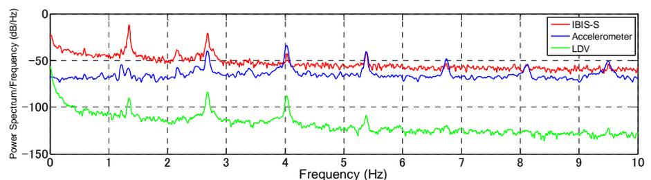
Figure 6. Comparison of power spectrum of measurement data
