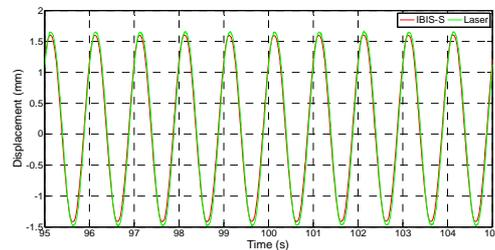
Figure 1. Comparison between the radar and laser sensor
