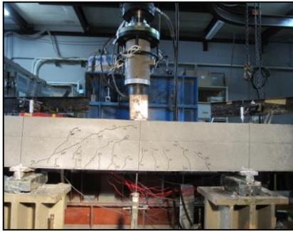
Fig.2 Crack pattern of B1
