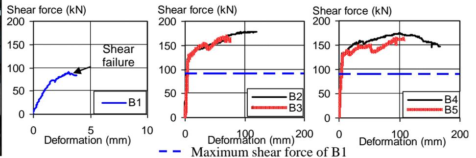
Fig.3 Shear force and deformation of B1-B5
