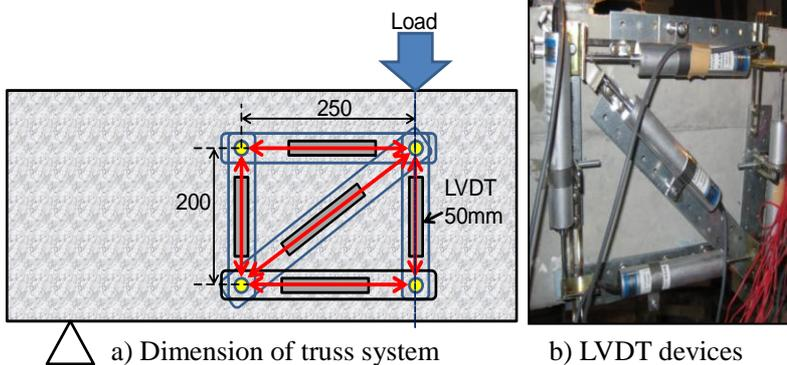
Fig.4 Truss mechanism
