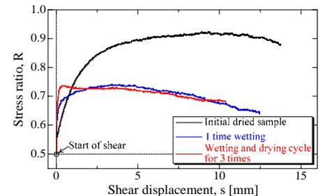
Fig. 4  $R$ - $s$  relationship under different test condition for  $R = 0.5$
