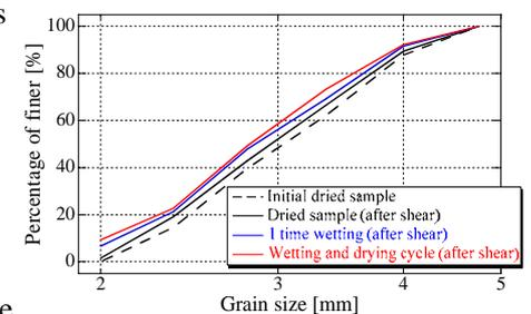
Fig. 5 Particle size distribution before and after experiment
