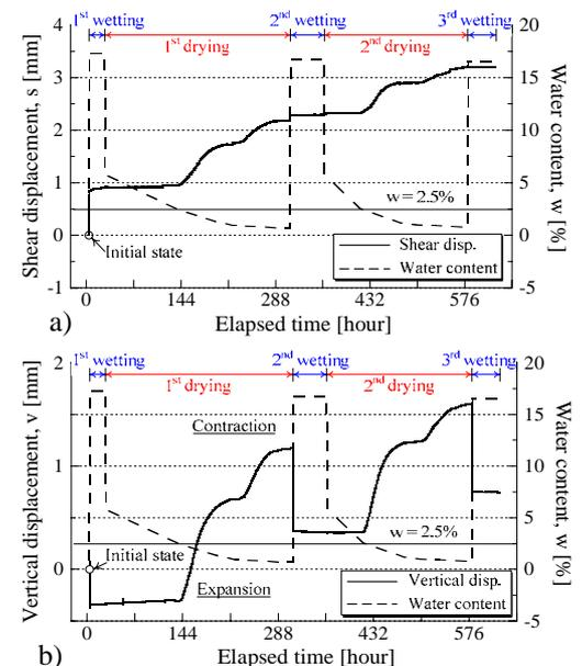
Fig. 1 Time histories of  $w$ ,  $s$  and  $v$  (a)  $s$  (b)  $v$  under cyclic W/D for 3 times for  $R=0.5$
