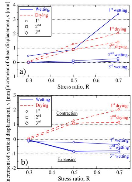
Fig. 2 Increment value of creep
