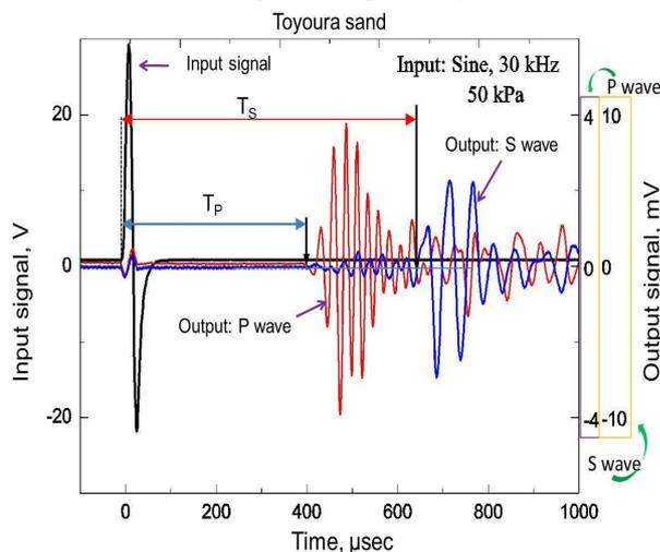
Fig.3 Typical P and S waveforms obtained on Toyoura sand
