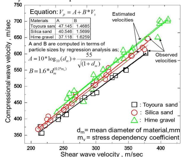
Fig. 4 Compressional and shear (P & S) waves velocities
