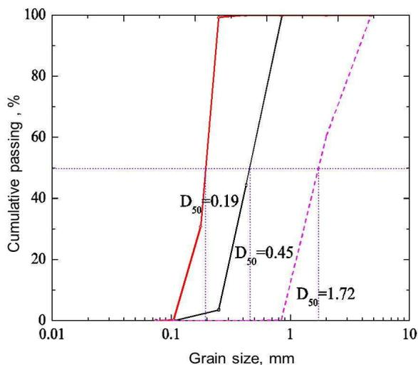
Fig.1 Particle size distribution curve of tested materials
