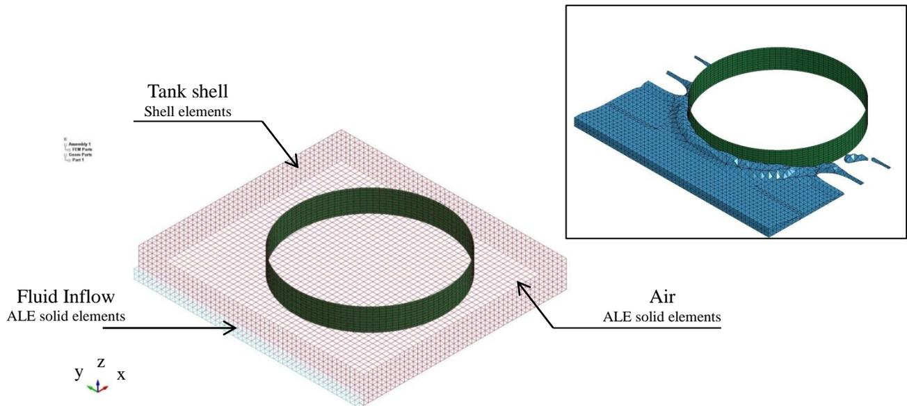
Fig. 1 Finite element domain for the analysis and deformed mesh during the simulation
