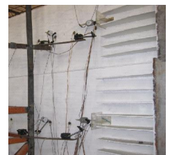
Fig. 6 Distribution of strain gauge in middle plate
