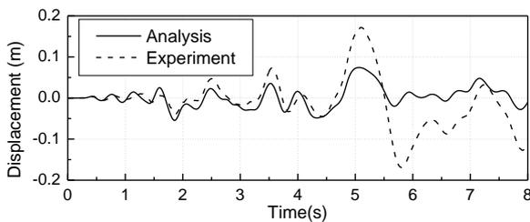
Fig. 4 Displacement time-history of RC pier in longitudinal direction
