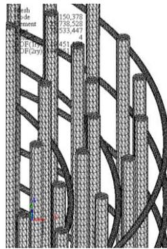
Fig. 1 FE model of RC pier Fig. 2 FE model of rebars
