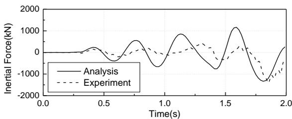
Fig. 5 Inertial force time-history of RC pier in longitudinal direction
